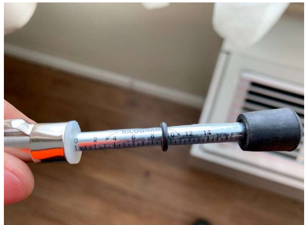
Photo 24 – Force required to open door
