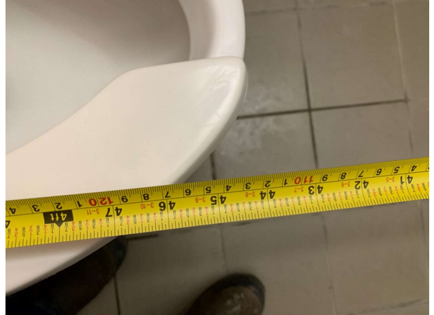
Photo 44 – Clear turning space diameter within the stall
