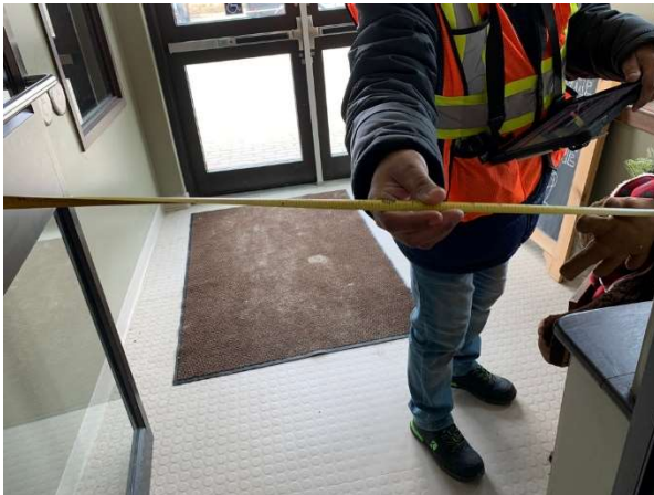
Photo 17 – Inner Door: Clear width of open door
