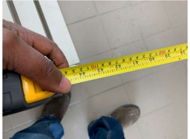
Photo 32 – Station Lobby – Path of Travel – Clear width (close-up measurement)
