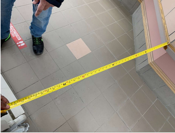
Photo 31 – Station Lobby – Path of Travel – Clear width
