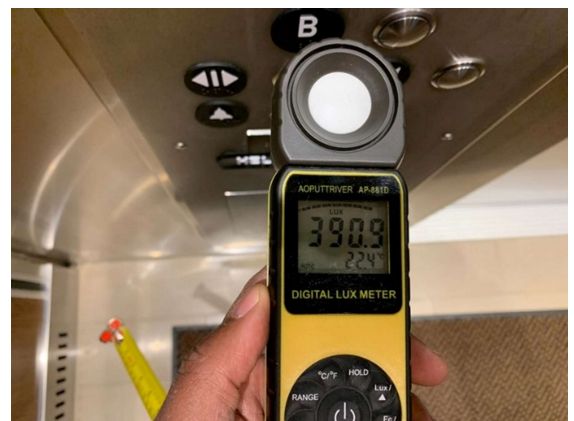
Photo 90 – Luminance at the car controls
